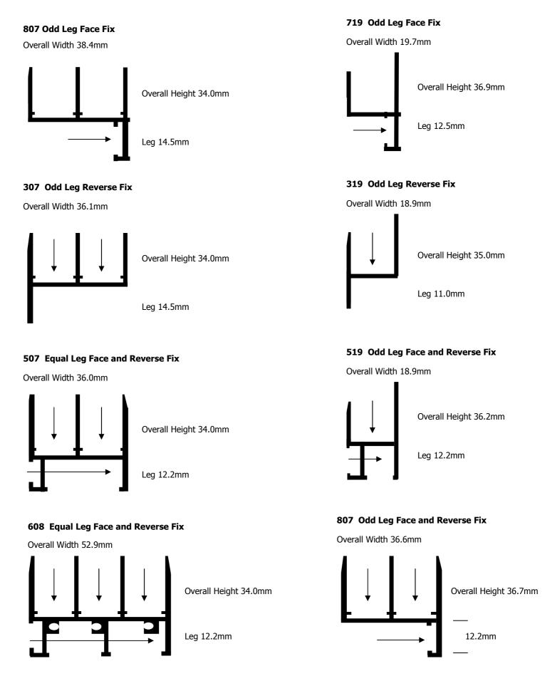
Arrows show direction of fixing screws. Arrows shown in two different directions section can be fitted either way Drawings are for illustration only. Do not scale
